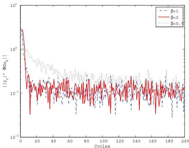
Fig. 2. Norm of the modified tracking error  $\|y_r - \Phi G u_k\|$  with different learning gain. [Color figure can be viewed at wileyonlinelibrary.com]
