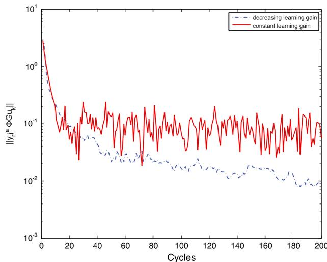
Fig. 1. Norm of the tracking error  $\|y_r - \Phi G u_k\|$ . [Color figure can be viewed at wileyonlinelibrary.com]
