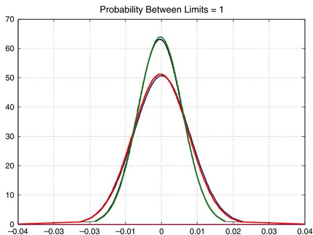
Fig. 5. The probability distribution function based on tracking error data at reference points. [Color figure can be viewed at wileyonlinelibrary.com]
